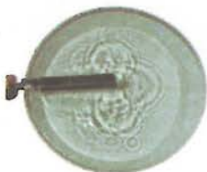
Fig. 10.4: (c) A prong of vibrating tuning fork touching the surface of water
