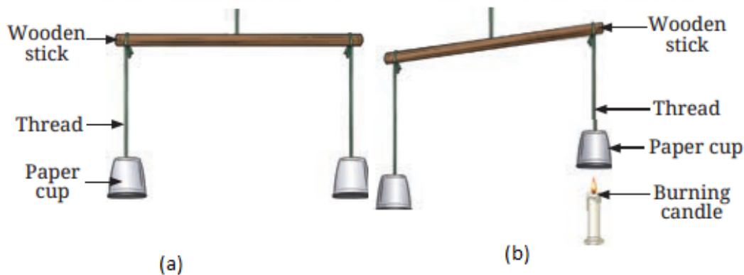
Fig. (a): Initial set-up (b): Hot air rising up
