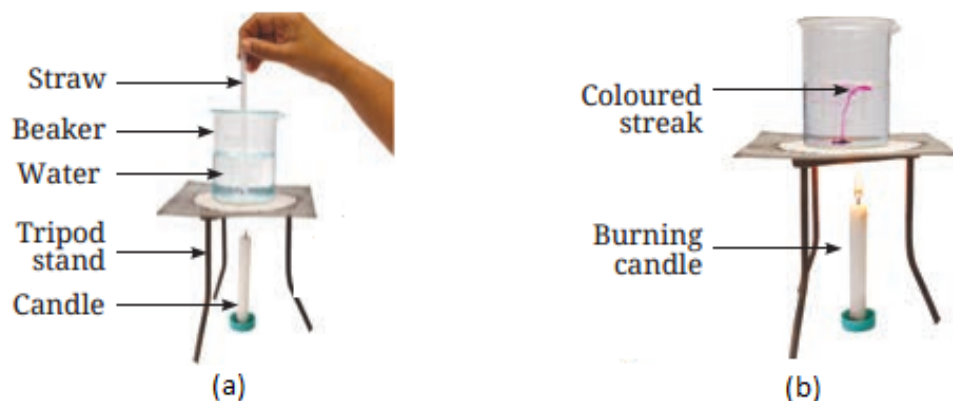
Fig. (a): Initial set-up for demonstration (b): Demonstration of convection in heated water
