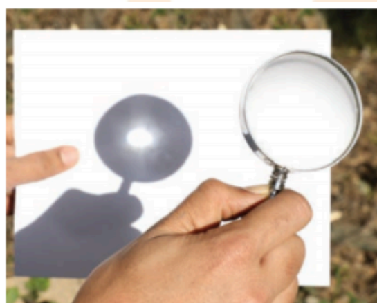
Fig. (a): Focusing the sunrays using a magnifying glass
