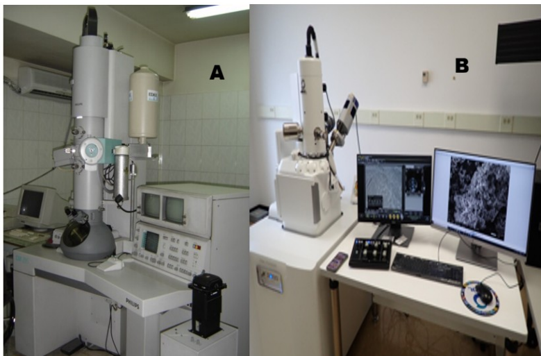
Figure 9.6: A. Transmission Electron Microscope B. Scanning Electron Microscope
