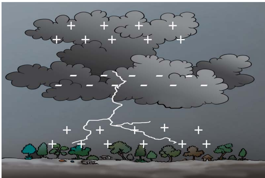
Fig. 12.5 : Accumulation of charges leading to lightning.
