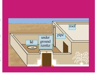
Some people collect rain water. This is done by a special method called Rain Water Harvesting – by making **tanks** (*tanka*). Do you know, what a *tanka* is and how is it built?
