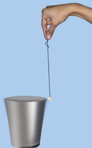
Fig. 10.17 : Thermocol ball touching the vibrating glass tumbler
