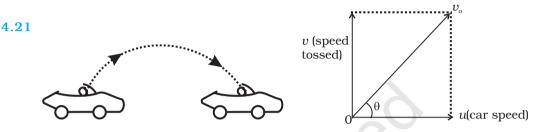
For a ground-based observer, the ball is a projectile with speed  $v_{o}$  and the angle of projection  $\theta$  with horizontal in as shown above.
